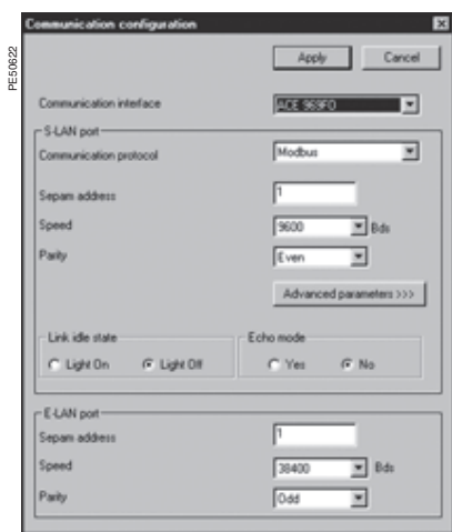
SFT2841: communication configuration window for ACE969FO.
