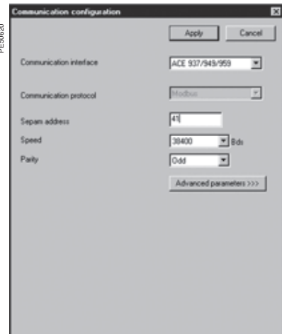
SFT2841: communication configuration window for ACE949.
